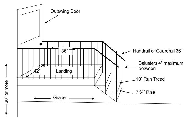
**Guardrail details.** Porches, balconies or raised floor surfaces located more than 30 inches (762 mm) above the floor or grade below shall have guardrails not less than 36 inches (914 mm) in height. Open sides of stairs with a total rise of more than 30 inches (762 m) above the floor or grade below shall have guardrails not less than 34 inches (864 mm) in height measured vertically from the nosing of the treads.
